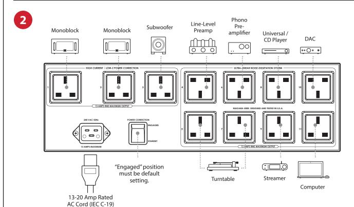
**Note:** Outlets 4 through 11 are subject to many variables and circuit conditions, so experimentation for best results is encouraged. Power amplifiers **must** be connected to Outlets 1 through 3.
