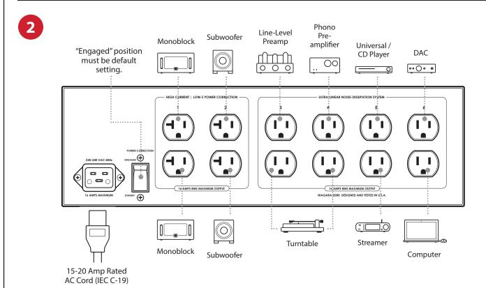
**Note:** Banks 3 through 6 are subject to many variables and circuit conditions, so experimentation for best results is encouraged. Power amplifiers **must** be connected to Banks 1 or 2.
