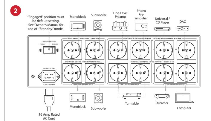
**Note:** Banks 3 through 6 are subject to many variables and circuit conditions, so experimentation for best results is encouraged. Power amplifiers **must** be connected to banks 1 or 2.
