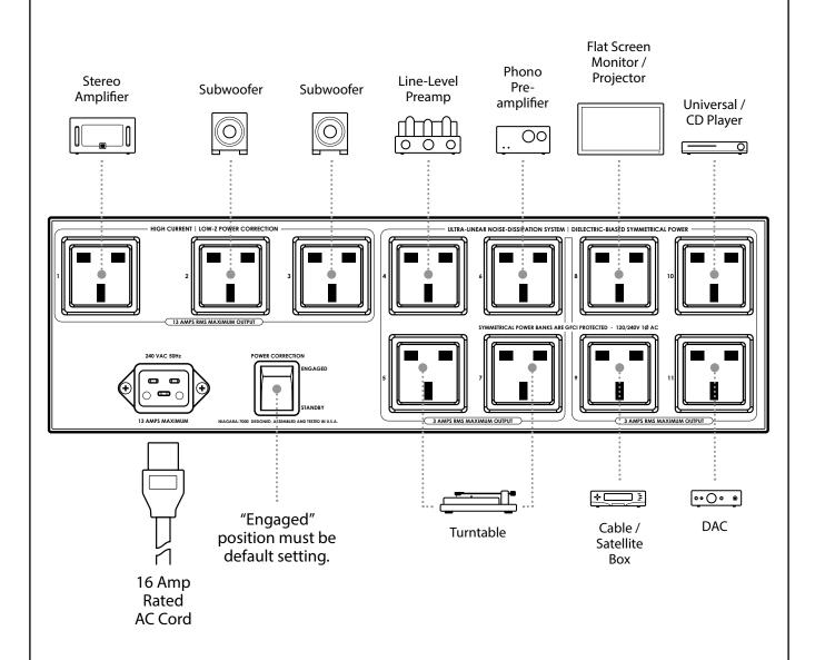
**Note:** Outlets 4 through 11 are subject to many variables and circuit conditions; experimentation is encouraged for best results. Power amplifiers **must** be connected to Outlets 1 through 3.
