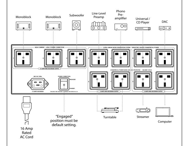
**Note:** Outlets 4 through 11 are subject to many variables and circuit conditions; experimentation is encouraged for best results. Power amplifiers **must** be connected to Outlets 1 through 3.
