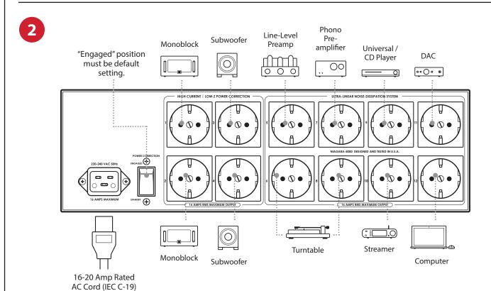
**Note:** Outlets 5 through 12 are subject to many variables and circuit conditions, so experimentation for best results is encouraged. Power amplifiers **must** be connected to Outlets 1 through 4.
