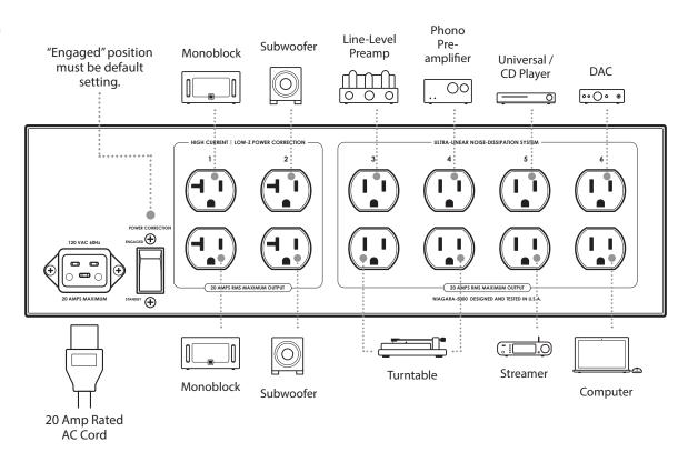
**Note:** Banks 3 through 6 are subject to many variables and circuit conditions, so experimentation for best results is encouraged. Power amplifiers **must** be connected to Banks 1 or 2.
