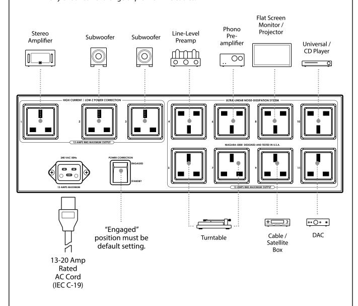
**Note:** Outlets 4 through 11 are subject to many variables and circuit conditions; experimentation is encouraged for best results. Power amplifiers **must** be connected to Outlets 1 through 3.
