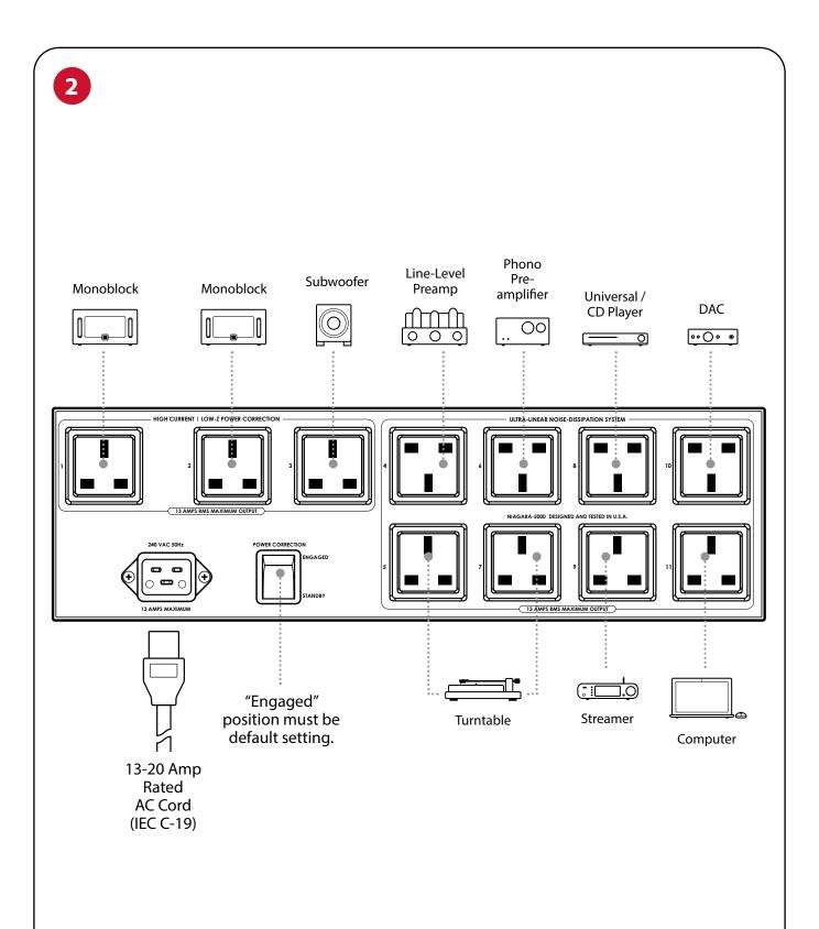
**Note:** Outlets 4 through 11 are subject to many variables and circuit conditions; experimentation is encouraged for best results. Power amplifiers **must** be connected to Outlets 1 through 3.
