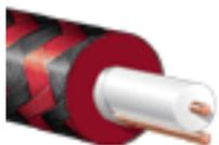
**AudioQuest Sidewinder** uses two solid LGC copper conductors in a novel symmetrical Hyperlitz arrangement. One conductor is insulated and used for positive. The other is uninsulated and makes contact with the 100% coverage shield, allowing it to connect (drain) the shield while at the same time being used as a high quality conducting path for the negative signal. This mild red jacketed cable carries a UL CL-3 rating, enabling it to be used inside walls without conduit.
