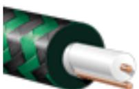
**AudioQuest Copperhead** uses two solid PSC copper conductors in the symmetrical Hyperlitz arrangement. One conductor is insulated and used for positive. The other is uninsulated and makes contact with the 100% coverage shield, allowing it to connect (drain) the shield while at the same time being used as a high quality conducting path.
