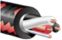
**AudioQuest Coral** is a Triple Balanced cable featuring Hyperlitz construction. Coral uses three solid PSC copper conductors, each insulated with foamed Polyethylene. When used single-ended (with RCA plugs), one conductor carries the positive audio signal, two carry the negative. The 100% coverage shield is only attached at one end so that it is not used as an inferior audio conductor.
